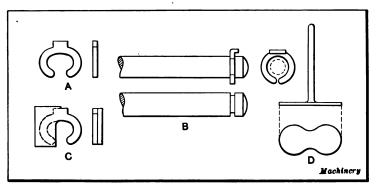
Fig. 9. Examples of Blanking Die Templets
